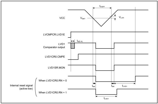
Figure 6.47 Timing of Voltage Detection by Voltage Monitoring Circuit 1 (V<sub>det1</sub>)
