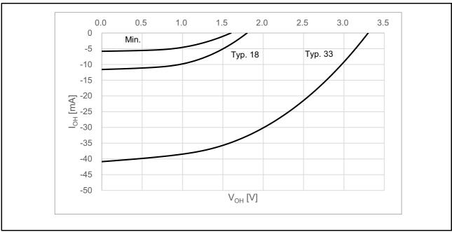
Figure 6.8 V<sub>OH</sub> vs. I<sub>OH</sub> Characteristics (High Driving Ability)
