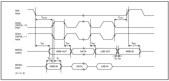
Figure 6.30 SCK Input and Output Timing (Simple SPI Mode) (Slave, SPMR.CKPH = 1)
