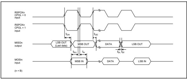
Figure 6.39 SPI Timing (Slave, CPHA = 1)
