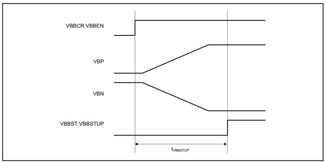
Figure 6.52 VBBC Initial Setup Timing
