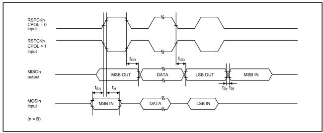
Figure 6.38 SPI Timing (Slave, CPHA = 0)
