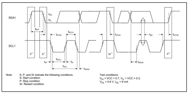
Figure 6.40 I<sup>2</sup>C Bus Interface Input and output Timing
