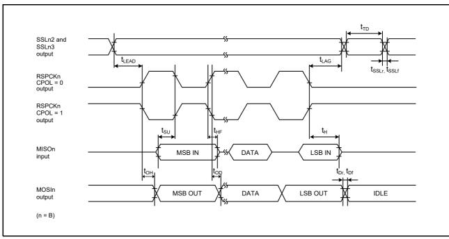
Figure 6.37 SPI Timing (Master, CPHA = 1) (Bit Rate: PCLKA Division Ratio is Set to 1/2)
