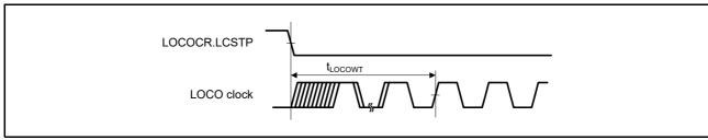
Figure 6.12 LOCO Clock Oscillation Start Timing
