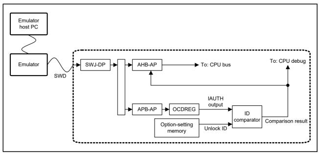
Figure 2.3 SWD Authentication Mechanism Block Diagram
