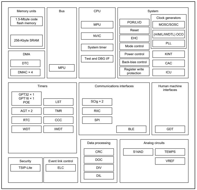
Figure 1.1 Block Diagram
