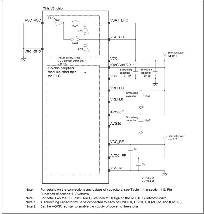
Figure B.1 Example of Connections for Normal Startup Mode
