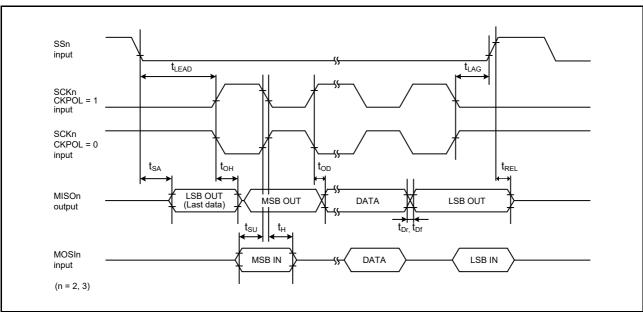
Figure 6.31 SCK Input and Output Timing (Simple SPI Mode) (Slave, SPMR.CKPH = 0)
