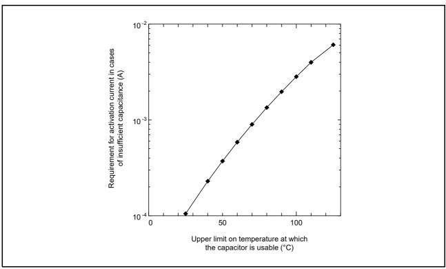
Figure 6.51 Relation between the Upper Limit of a Temperature and an Activation Current in the Case where Capacitance is Insufficient
