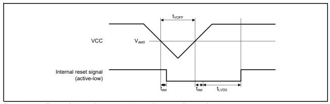
Figure 6.46 Timing of Voltage Detection by Voltage Monitoring Circuit 0 (V<sub>det0</sub>)
