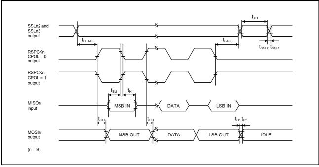
Figure 6.36 SPI Timing (Master, CPHA = 1) (Bit Rate: PCLKA Division Ratio is Set to Any Value Other than 1/2)
