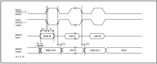
Figure 6.28 SCK Input and Output Timing (Simple SPI Mode) (Master, SPMR.CKPH = 1)
