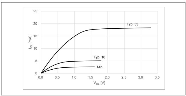
Figure 6.5 V<sub>OL</sub> vs. I<sub>OL</sub> Characteristics (Standard Driving Ability)
