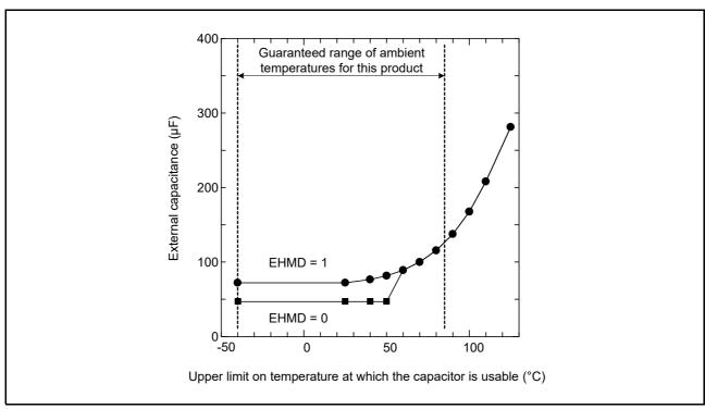
Figure 6.50 Relation between the Upper Limit on Temperature and Capacitance of the Storage Capacitor Connected to VCC\_SU
