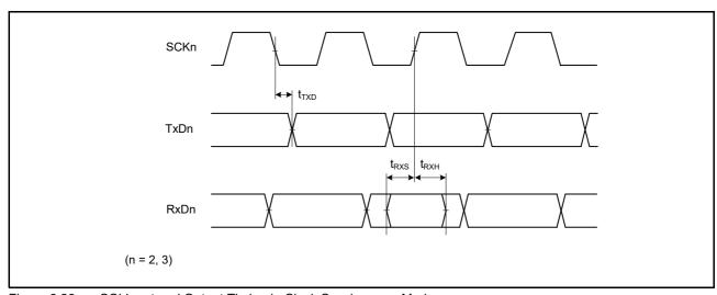
Figure 6.26 SCI Input and Output Timing in Clock Synchronous Mode
