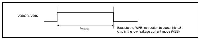
Figure 6.53 Internal Voltage Discharge Time
