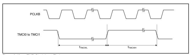
Figure 6.42 TMR Clock Input Timing
