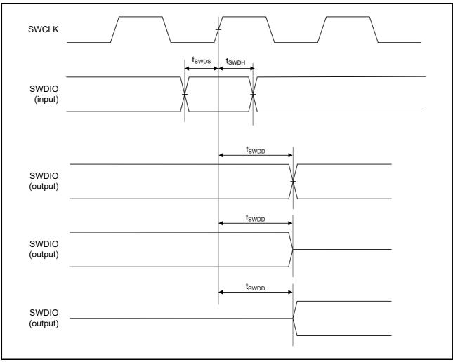
Figure 6.56 SWD Input and Output Timing
