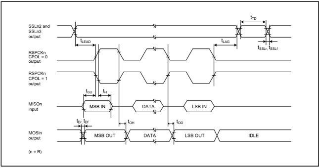
Figure 6.34 SPI Timing (Master, CPHA = 0) (Bit Rate: PCLKA Division Ratio is Set to Any Value Other than 1/2)
