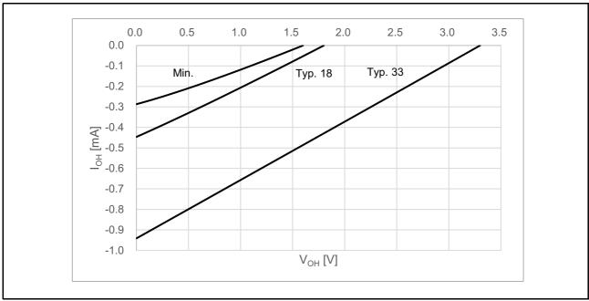
Figure 6.4 V<sub>OH</sub> vs. I<sub>OH</sub> Characteristics (Middle Driving Ability)
