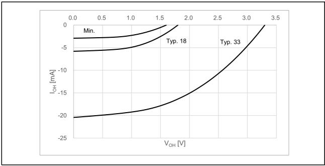
Figure 6.6  $V_{OH}$  vs.  $I_{OH}$  Characteristics (Standard Driving Ability)
