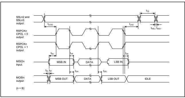
Figure 6.35 SPI Timing (Master, CPHA = 0) (Bit Rate: PCLKA Division Ratio is Set to 1/2)
