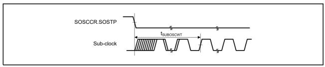
Figure 6.14 Sub-clock Oscillation Start Timing
