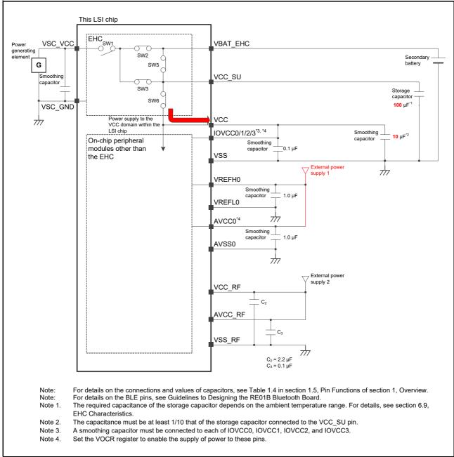
Figure B.5 Example of Connections in Energy Harvesting Startup Mode with Certain External Power Sources
