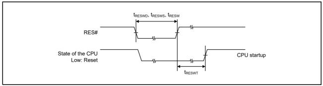
Figure 6.16 Reset Input Timing
