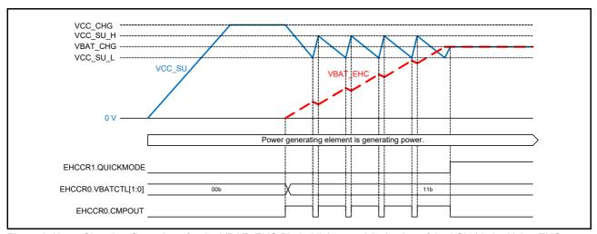
Figure 6.49 Charging Operations for the VBAT\_EHC Pin in High-speed Activation of the LSI chip by Using EHC Capacitor Charging
