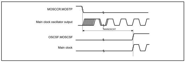
Figure 6.11 Main Clock Oscillation Start Timing
