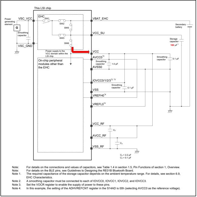
Figure B.3 Example of Connections in Energy Harvesting Startup Mode with AVCC0 as the Reference Voltage
