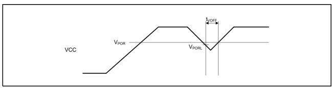
Figure 6.45 Power-on Reset Timing
