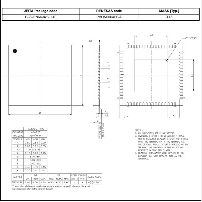
Figure A.1 64-Pin QFN (PVQN0064LE-A)
