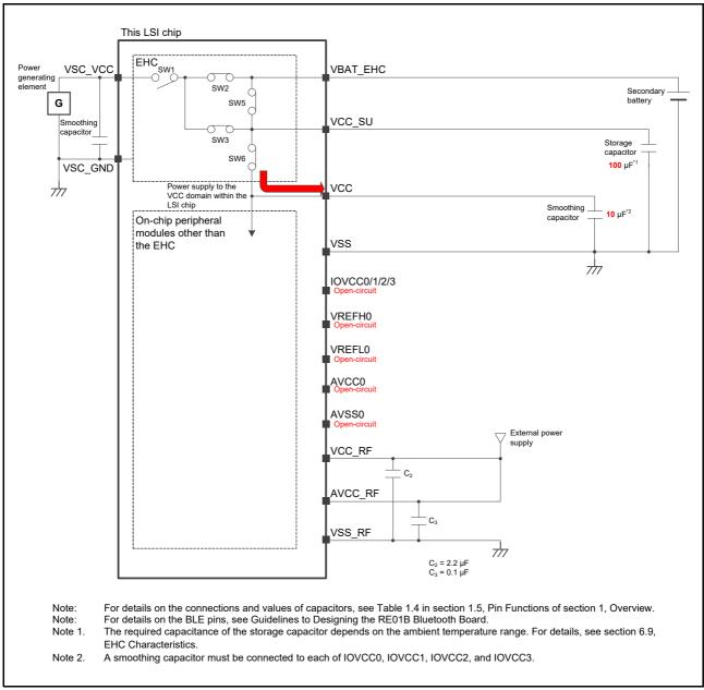
Figure B.6 Example of Minimum Connections in Energy Harvesting Startup Mode
