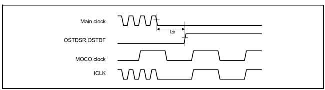
Figure 6.44 Oscillation Stop Detection Timing
