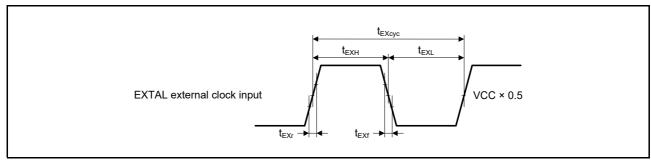
Figure 6.10 EXTAL External Clock Input Timing
