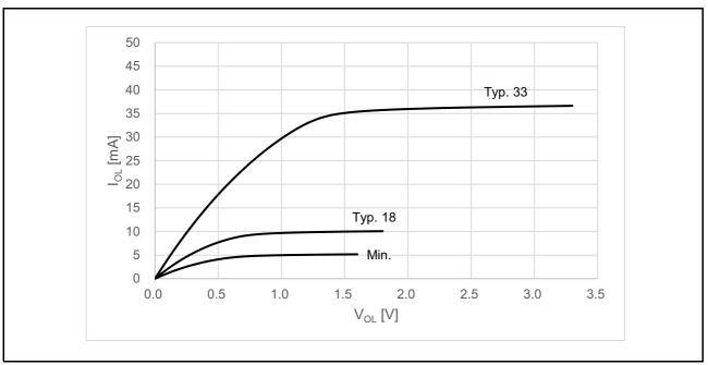
Figure 6.1 V<sub>OL</sub> vs. I<sub>OL</sub> Characteristics (Low Driving Ability)
