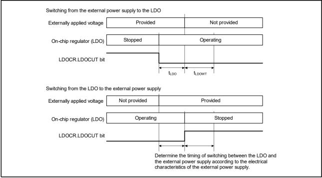
Figure 6.9 Timing of Switching between the External Power Supply and the LDO
