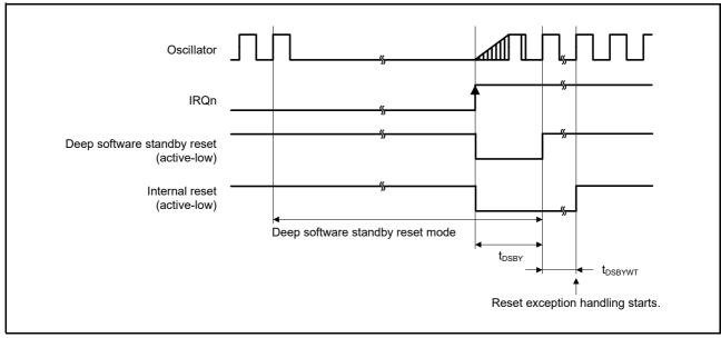
Figure 6.17 Timing of Release from Deep Software Standby
