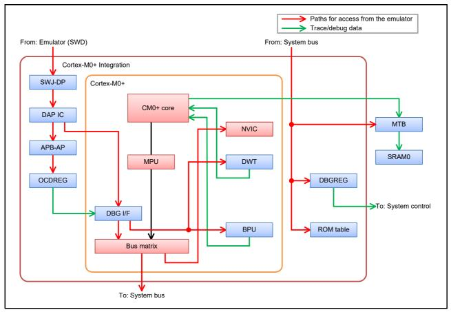
Figure 2.1 Cortex-M0+ CPU Block Diagram
