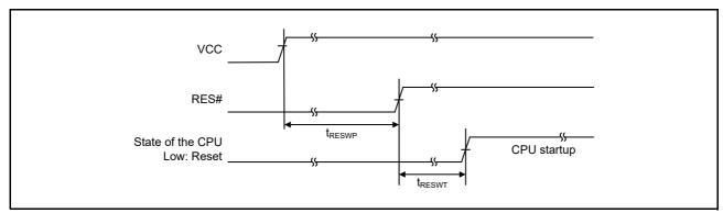
Figure 6.15 Timing of Input through the Reset Pin when Power is Supplied
