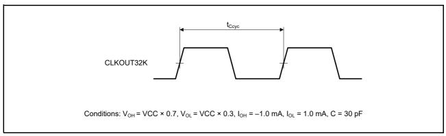
Figure 6.41 CLKOUT Output Timing
