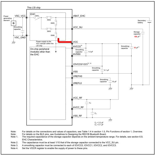
Figure B.4 Example of Connections in Energy Harvesting Startup Mode with the VREF in Use (2)
