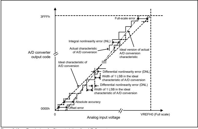
Figure 6.43 Terminology for Characteristics of an A/D Converter
