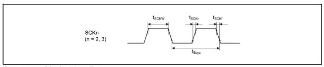
Figure 6.25 SCK Clock Input Timing
