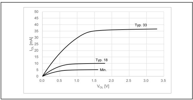
Figure 6.3 V<sub>OL</sub> vs. I<sub>OL</sub> Characteristics (Middle Driving Ability)
