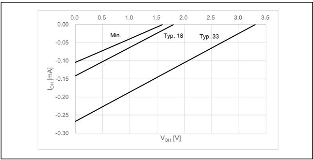
Figure 6.2 V<sub>OH</sub> vs. I<sub>OH</sub> Characteristics (Low Driving Ability)
