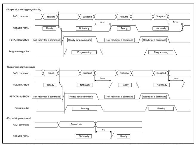
Figure 6.54 Timing of Suspension during Programming and Erasure and Timing of Forced Stop of the Flash Memory
