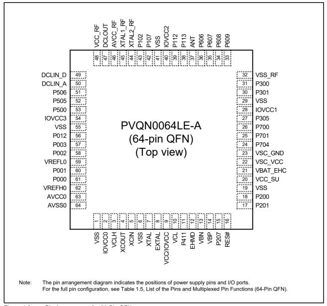
Figure 1.2 Pin Arrangement for 64-Pin QFN
