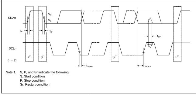
Figure 6.32 SCK Input and Output Timing (Simple I<sup>2</sup>C Mode)
