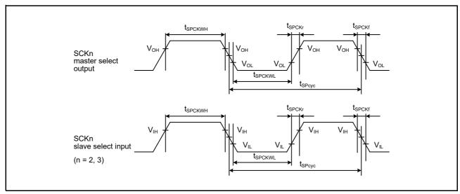
Figure 6.27 SCK Clock Input and Output Timing (Simple SPI Mode)
