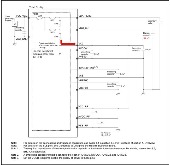
Figure B.2 Example of Connections in Energy Harvesting Startup Mode with the VREF in Use (1)
