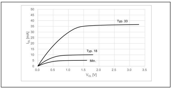
Figure 6.7 V<sub>OL</sub> vs. I<sub>OL</sub> Characteristics (High Driving Ability)
