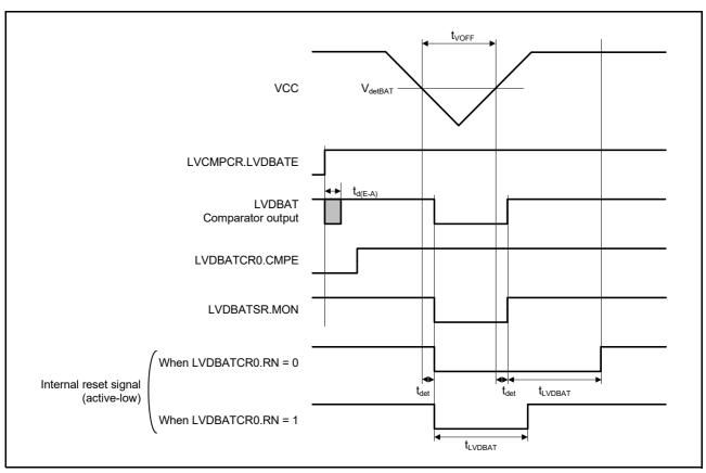
Figure 6.48 Timing of Voltage Detection by Voltage Monitoring BAT Circuit (V<sub>detBAT</sub>)
