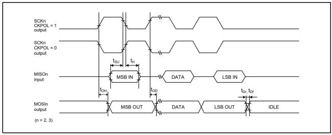
Figure 6.29 SCK Input and Output Timing (Simple SPI Mode) (Master, SPMR.CKPH = 0)
