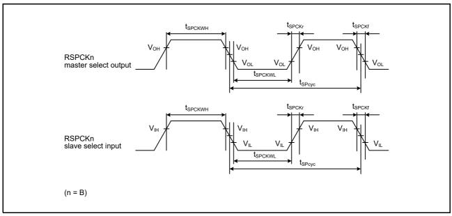
Figure 6.33 SPI Clock Timing
