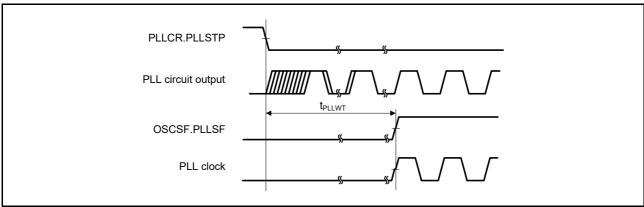
Figure 6.13 PLL Clock Oscillation Start Timing
