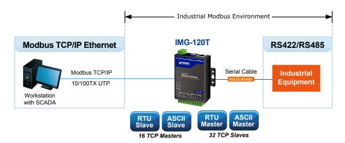
The advantage of having the IMG-120T is to assist users to build an industrial environment between the Modbus TCP/IP Protocol and the Modbus RTU/ASCII Protocol easily, thus offering an application solution to the industrial control equipment without Ethernet ports. Thus, the industrial control equipment can only control through an industrial PC workstation or industrial control panel.
