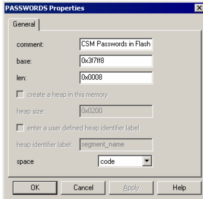
Figure 3. DSP/BIOS MEM Properties for CSM Password Locations
